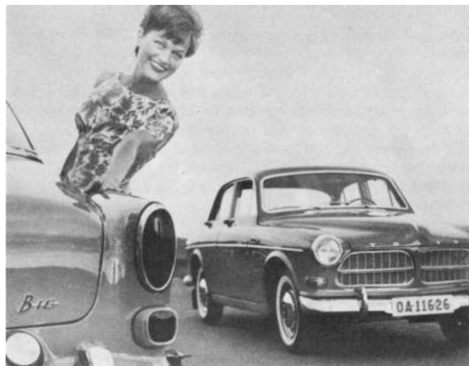
The B-18 symbol of the rear trunk lid and front grill identify this as a new 90 h.p. B-18 Series Volvo. Other exterior changes on the 122-S shown above include a narrower center post and wider front grill mesh for more rapid cooling, and addition of an amber directional flasher in combination with the front parking lights.
