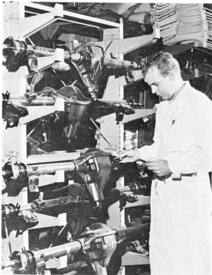
Rear axle units also receive special treatment at Volvo warehouses. Use of these special racks not only aids in handling and storage, but also prevents corrosion which might occur if the units were stored on floors or shelves on which the protective coatings in which they are shipped could be rubbed off.
