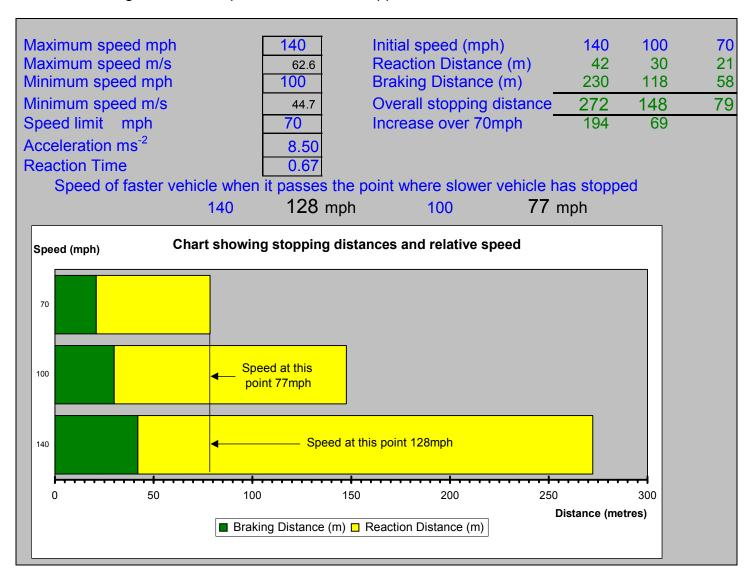
This graphic illustrates the same information but the rate of deceleration used is 4ms<sup>-2</sup>. This would represent the sort of deceleration that might be achieved on a wet road surface. It should be noted that, compared to the previous example the overall stopping distance at a speed of 140mph more than doubles.
