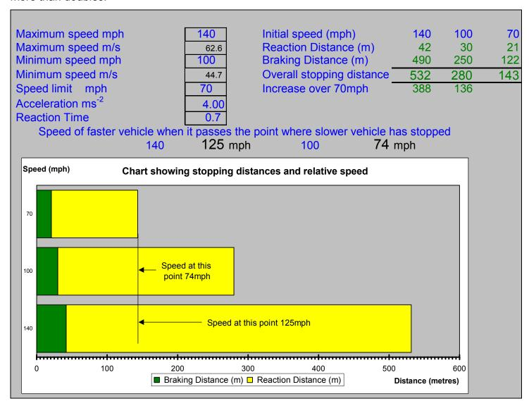
These figures will apply to all vehicles. However, as with all such calculations, some variations will occur. More modern technology such as Active Chassis and STDC fitted to top range cars will have some affect on the figures, as will modifications to braking systems, such as the fitting of AP brakes. In the end, physics will be the over riding master, so these figures will probably not change much more than about 10%.
