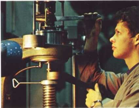
Hardened safety components such as, for example, king pins and spring bolts, are subjected to extensive control in a hardness test.
