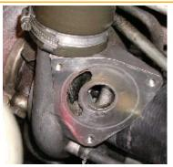
**Replacement Diaphragms for CBV**. Various turbo rebuilders carry the diaphragm repair kits for reasonable prices. Check Rick Banas at D&W Diesel (r.banas@dwdiesel.com) for Mitsu diaphragms and some Garretts.
