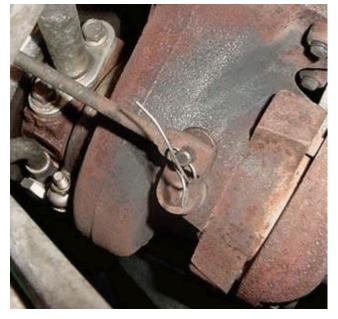
below and use a Dremel tool with a right-hand drill attachment. Be prepared to use up about five or six titanium 1/16 inch bits on this very hard rod. Replace it with a new clip, a stainless cotter pin, or a piece of stainless wire. If the rod is too tight to pull back onto the stem, just unbolt the actuator, secure the rod, and re-bolt.
